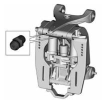
Use a grease gun and fill up with recommended grease until the grease comes out at the joints or ends of shaft.Refer to *Recommended fluids and* grease. 2. Fill the seatings with grease for smoother tilt operation. Use grease according to *Recommended fluids and grease*.
