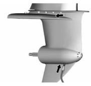
Alternatively, use an oil filling device and fill up the oil through the oil plug hole (2) until oil comes out at oil plug hole (1).
