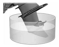
Run the outboard until the entire sea-water part of the system is filled with coolant fluid and thus protected from freezing and corrosion.
