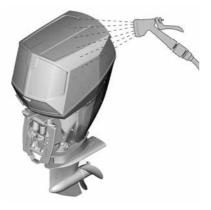
Flush the outside of the outboard with fresh water and, if possible, flush the power head under the cowling. 2. Drain the cooling seawater completely out of the engine.
